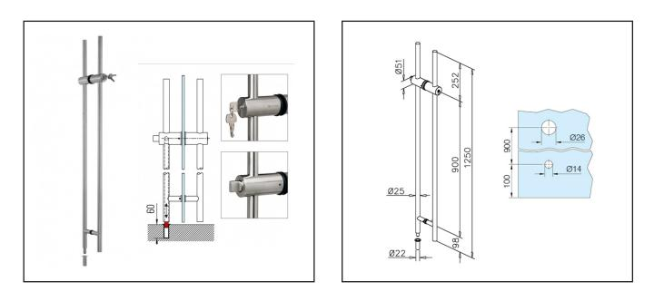
**Product Specification** A pull handle set for glass doors, with integrated locking mechanism Includes the specific euro cylinder & keys
