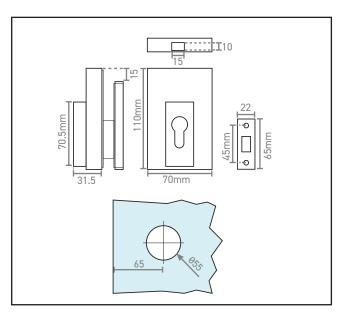
**Product Specification** With a glass free edge, this deadlock is suitable for glass doors in frames Double throw function Takes a standard euro profile cylinder Strike Plate included with screws
